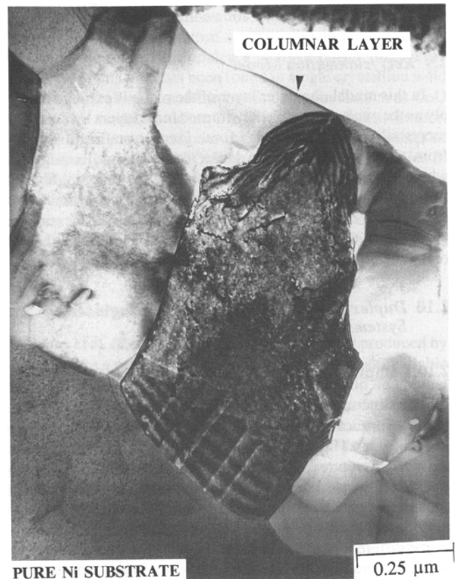
Fig. 9 Transverse section image of TEM of a 5 min oxidation scale grown at 1273 K in air on the pure Ni substrate, showing the oxide layer composed of a single columnar layer
